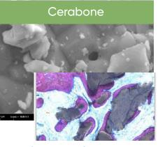
\*Equivalent material sintered at 1200C
