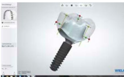
7 | The fine tuning of the abutment design should be based on the preparation guidelines for natural teeth, as well as on the guidelines for the materials being used.
