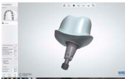
8 | The final individual CAD-designed abutment with virtual TitaniumBase.
