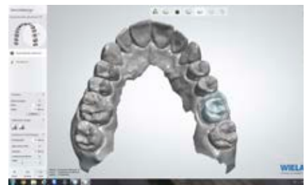
6 | The abutment is designed based on the desired final crown shape.
